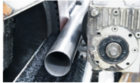
Centerless grinding of tubes and bars
