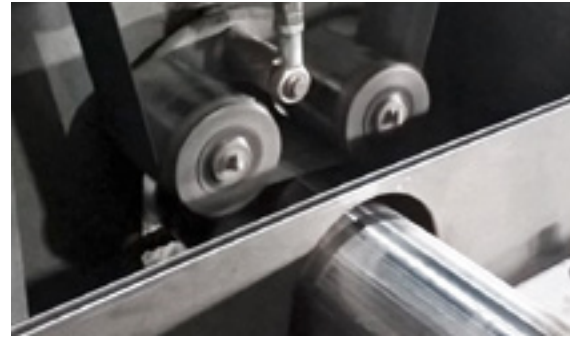
Grinding of longitudinally welded tubes
