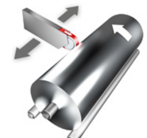
Cylindrical grinding of rollers during roller pass
