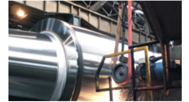
Cylindrical grinding of rollers during roller pass
