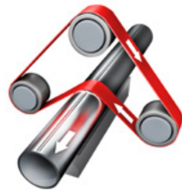
Grinding of longitudinally welded tubes
